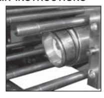
8) Take out the seal case (38) from the valve (if necessary secure 2 screwdrivers in the front O-ring groove to extract seal casing from valve casing). Coat seals with silicon grease before installing.
